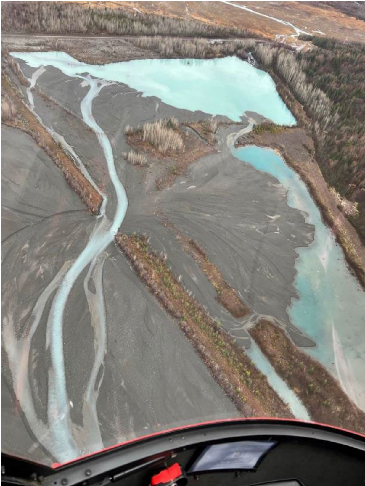
Photo 3-2 Extent of Deposition in Mitigation Ponds; New Martin River Outlet to Tidewater (top right) November 2, 2023.
